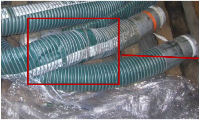
Displaced outer wire is usually the result of over bending
