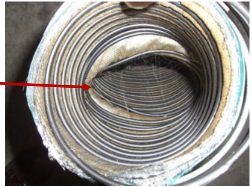
Hose cut and ID exposed showing inner wire movement
