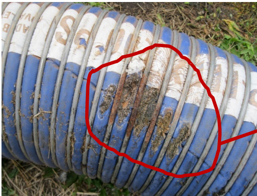
Severe cover abrasion
