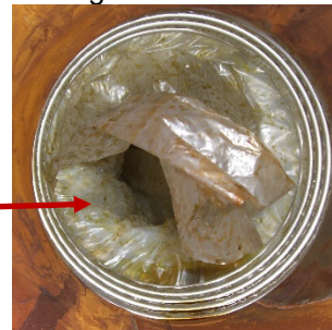
View looking in from coupling Inner wire has rolled/moved
