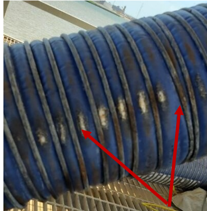
Abrasion through the cover with outer wire displacement
