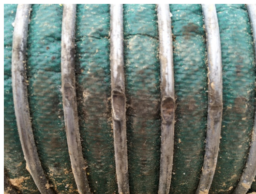
Severe wire abrasion/cutting
