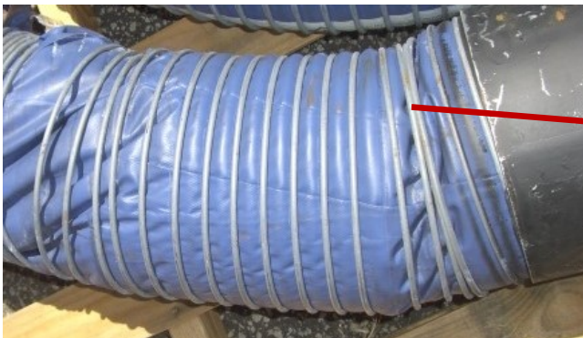
Damage from over bending
