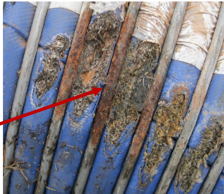
Abrasion through the cover with outer wire displacement
